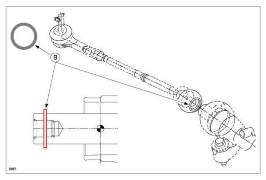
6. Install the tie rod assembly (both sides) according to the instructions on MGSS online (STEERING GEAR AND LINKAGE ASSEMBLY - Tie Rod Assembly Note).
