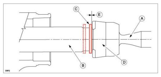
7. Reinstall the boot using a new boot band from the joint set (both sides) according to the instructions on MGSS online (STEERING GEAR AND LINKAGE ASSEMBLY - Boot Band Assembly Note).
