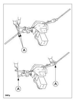
5. Install the driver side spacer (A) and passenger side spacer (B) onto the steering rack bar as shown below.
