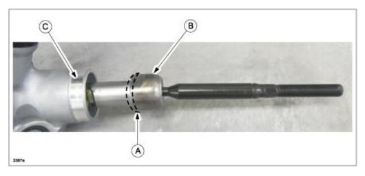
To eliminate the noise, a spacer (A) has been installed between the inner ball joint (B) and the steering gear housing (C) (both sides) to prevent direct contact.
