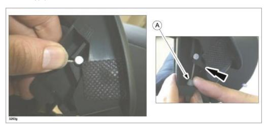
2. Engage the hook (A) at the front of the lever with the anchor (B) from the seat frame.
