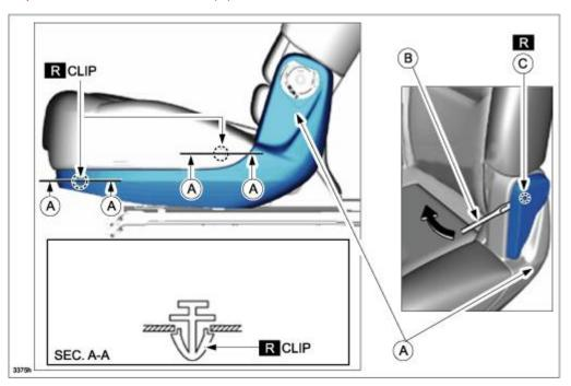
8. Inspect cable bracket (A) for bending.
