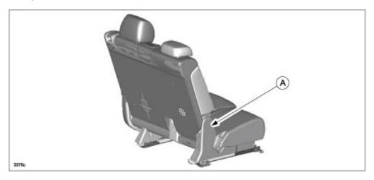
5. Inspect the cable bracket (A) for deformation / bending.
