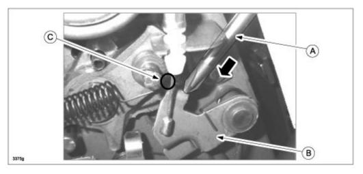
7. Using a screwdriver (B), remove the side cover (A) (driver-side/rear door-side second-row seat) according to the instructions on MGSS online (SECOND-ROW SEAT SIDE COVER REMOVAL/INSTALLATION → Driver-side second-row seat → Rear door-side second-row seat side cover). Replace the recliner lever knob (C) too.
