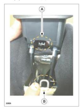
3. Push the lever assembly into the seat back, verifying that the front edge is securely engaged in the anchor.
