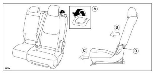
These concerns may be caused by a disconnected walk-in lever cable. To eliminate these concerns, the design of the walk-in lever has been changed according to the following:
