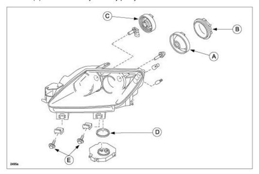
**NOTE:** LED headlamp assembly with LED turn signal lamp replacement part include seals. Seal transfer is not required.
