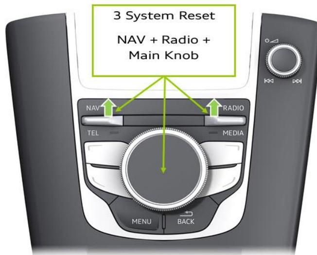
**Figure 5.** Three-finger system reset
