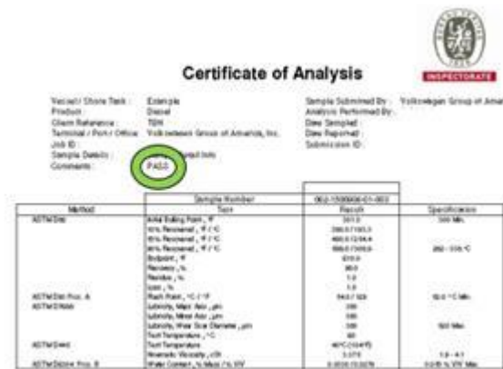
Figure 5. Example of a clean fuel sample analysis.
