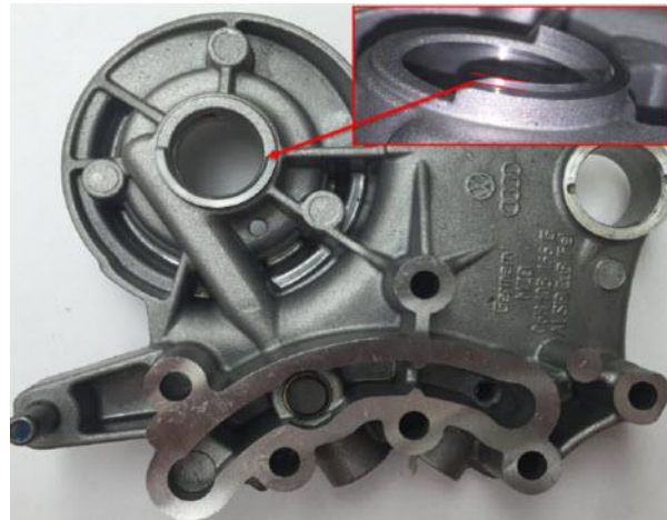
Figure 1. Worn thrust surface.
