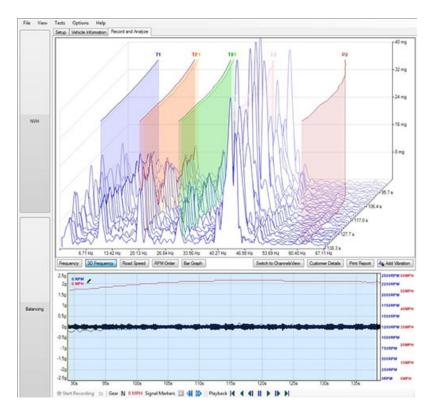
If TCC Shudder is present, a vibration peak will appear at approximately 43Hz +/-3Hz as shown in the picture above. If the vibration frequency follows engine, tire, or driveshaft speed, then it is NOT TCC Shudder. TCC Shudder vibration frequency should stay constant per gear while vehicle and engine speeds change.
