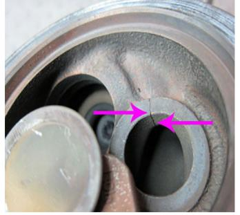
Wastegate solenoid valve port broken (replace solenoid valve - released for service)
