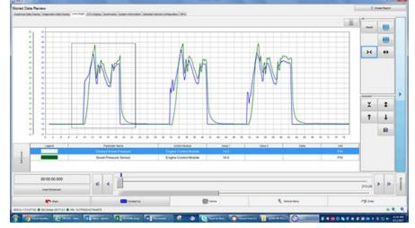
Example of normal turbocharger wastegate operation:
