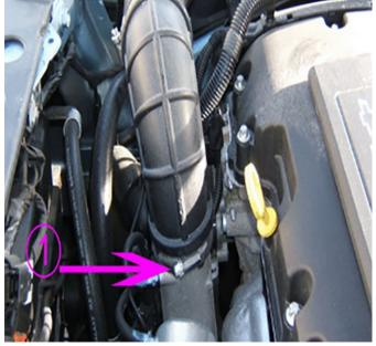
Notice: The view shown below indicates NORMAL oil staining in the turbocharger outside air inlet. This dry stain does not represent an oil leak.
