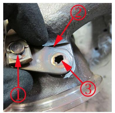
Disconnected wastegate lever arm pin (1) from the lever arm (crank) (2). Wastegate valve/linkage seized (cannot move).
