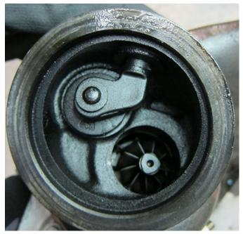
If oil is present in the exhaust system, then inspect the turbocharger turbine and compressor wheels to be sure that they are not broken off. It is very unlikely that the turbocharger will leak oil internally if the turbine and compressor wheel shaft is not broken. Refer to the current publication of <u>PIP5197</u> for diagnostic tips for oil coming through the exhaust ports or PCV system. CAC ICING and cold weather issues:
