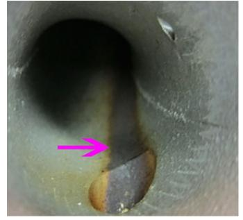
Inspect the inside of the turbocharger outside air inlet tube (3) for oil leaking into the opening of the turbocharger bore for the PCV bypass hose. Note: If oil is leaking into the opening; refer to the current version of <u>PIP5197</u>.
