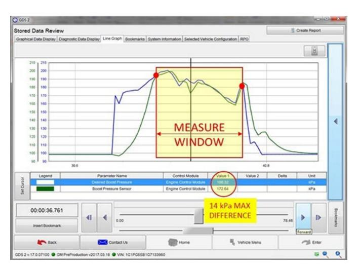
Example of a malfunctioning turbocharger wastegate:
