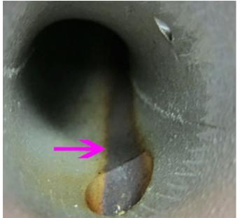
Inspect the inside of the turbocharger outside air inlet tube (3) for oil leaking into the opening of the turbocharger bore for the PCV bypass hose.
