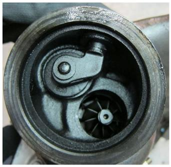
If oil is present in the exhaust system, then inspect the turbocharger turbine and compressor wheels to be sure that they are not broken off. It is very unlikely that the turbocharger will leak oil internally if the turbine and compressor wheel shaft is not broken.
