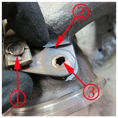
Disconnected wastegate lever arm pin (1) from the lever arm (crank) (2).
