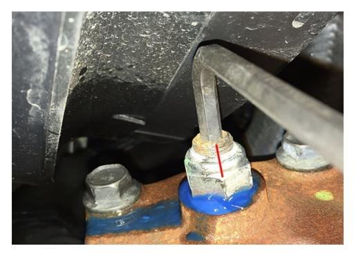
7. Using a torque wrench with crow foot & Allen wrench, turn the adjuster stud and nut simultaneously while torquing to 68 lb ft (92 Nm). Make sure the mark or scribe on the adjuster stud and nut (made during step 2) are still in alignment. If not, slightly loosen the nut, realign the marks, and retorque.
