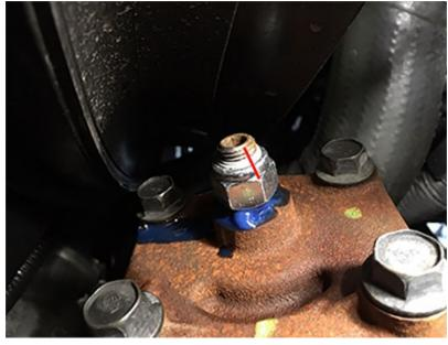
6. Using an Allen wrench, tighten the adjuster stud (turning clockwise) until the nut bottoms out on the cover plate, shown below.
