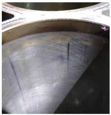
Shown below is an example of a damaged cylinder wall.
