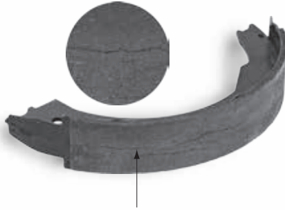
Acceptable Hairline Cracks
