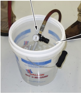
ATF WARMER PRESSURE TEST
