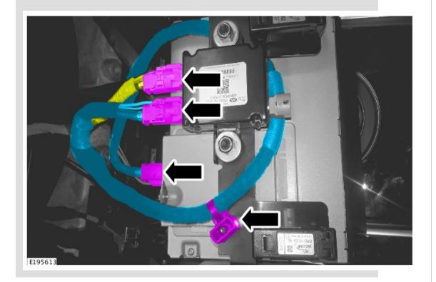
Connect the pink and yellow link lead harness connectors (taped together in Step 7) into the USB 2.0 hub.
