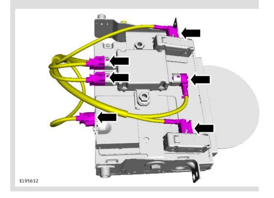
Disconnect the electrical connectors from the digital disc player, USB 2.0 hub, and Wi-Fi/Bluetooth $^{\text{TM}}$  antennas.
