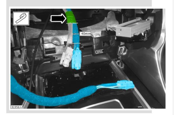
Tape the new link lead yellow connector alongside the pink connector on the Instrument Panel (IP) harness.
