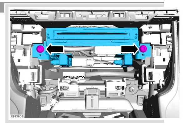
Remove the digital disc player and withdraw the unit to view the wiring harness connections.
