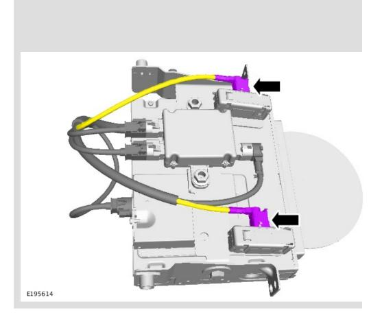
Connect the two remaining leads to the Wi-Fi/Bluetooth  $\mbox{\footnotember{$^{\top}$}}{}$  antennas.
