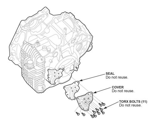
5. Replace the cover, the sealing gasket, and bolts with the new ones from the kit. Torque the bolts to **10.0 N-m (7 lb-ft)** in the sequence shown.
