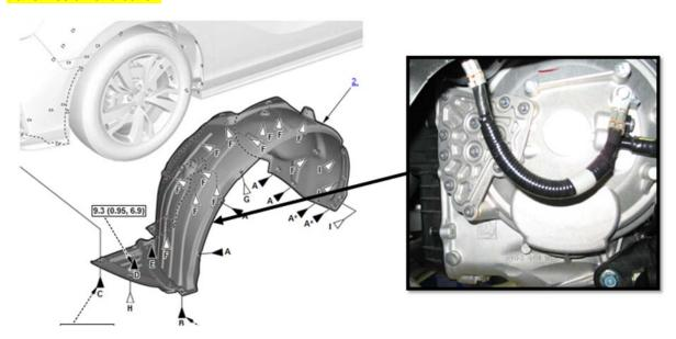
3. Pilot only. Loosen the front of the inner fender to access the transmission end cover.
