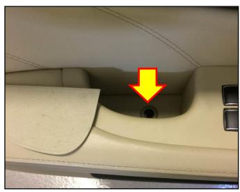
1C. Use a small and short Phillips screwdriver, remove the plastic screw and then pull the locking tab out.
