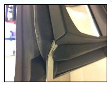
Separate the top trim cover, disconnect the tweeter connector, and remove it from the door panel.
