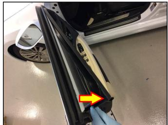
To remove the door panel, gently pull the door trim cover away from the door frame.
