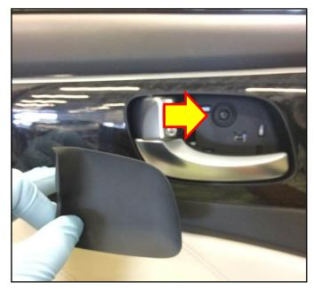
1B. Use a small flathead screwdriver, lift and remove the door pocket cover.
