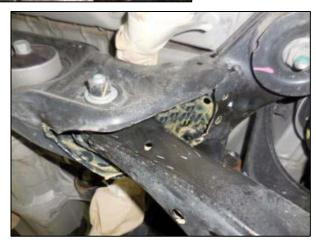
6. Rear lower control arms – Interior surfaces (using "inside" nozzle)
