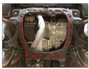
Front cross member (rear side of cross member, blowing air towards the front of the vehicle)
