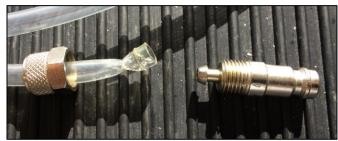
2b. Attach the compression fitting to the tubing on the new nozzle assembly.
