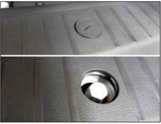
3. Remove the spare wheel/tire assembly.
