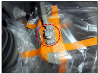
6. Wrap large plastic bags around the wheel/tire/brake assemblies to protect them from overspray. Use tape to secure the plastic in place.
