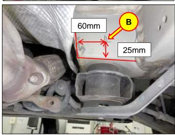
11. Center punch at positions A and B, as previously measured and marked.
