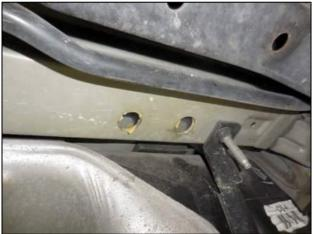
Service Procedure #4: Applying the Undercoating Spray
