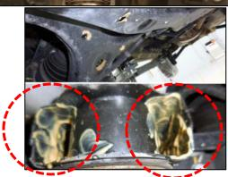
2. Front lower control arms – Interior surfaces (using *"inside"* nozzle)
