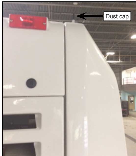
Figure 4 - Dust Cap of PRD Vent Pipe Location
