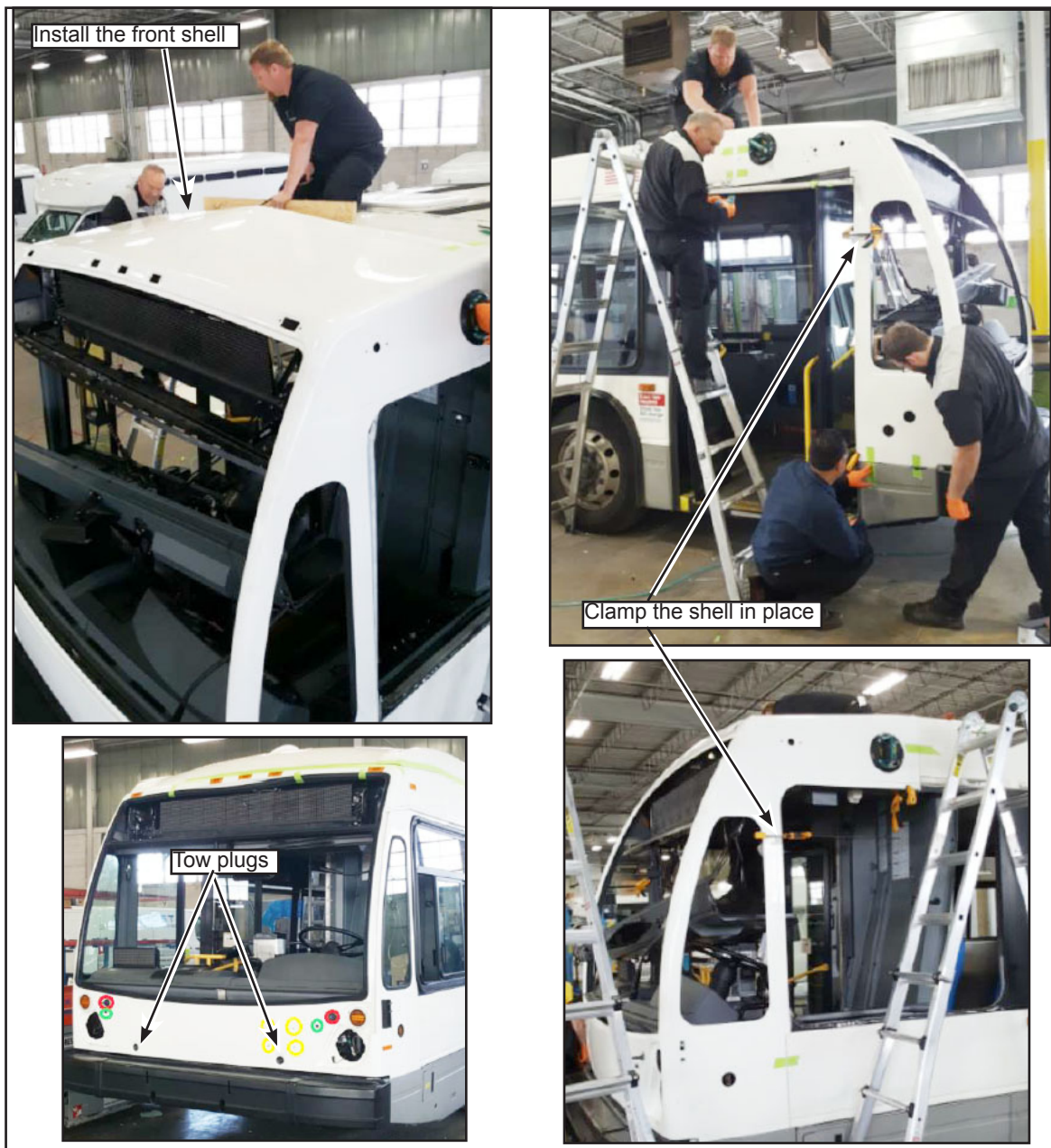
Figure 29 - Install the Front Shell
