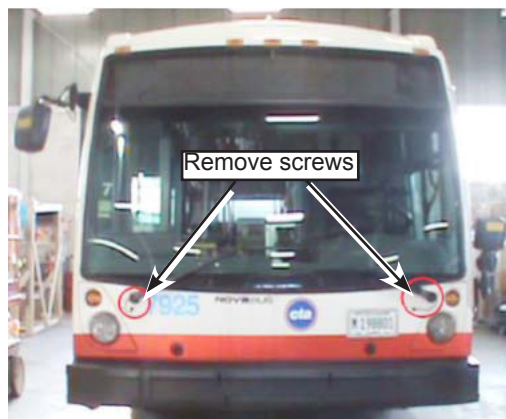
Figure 5 - Remove the Wiper Arms
