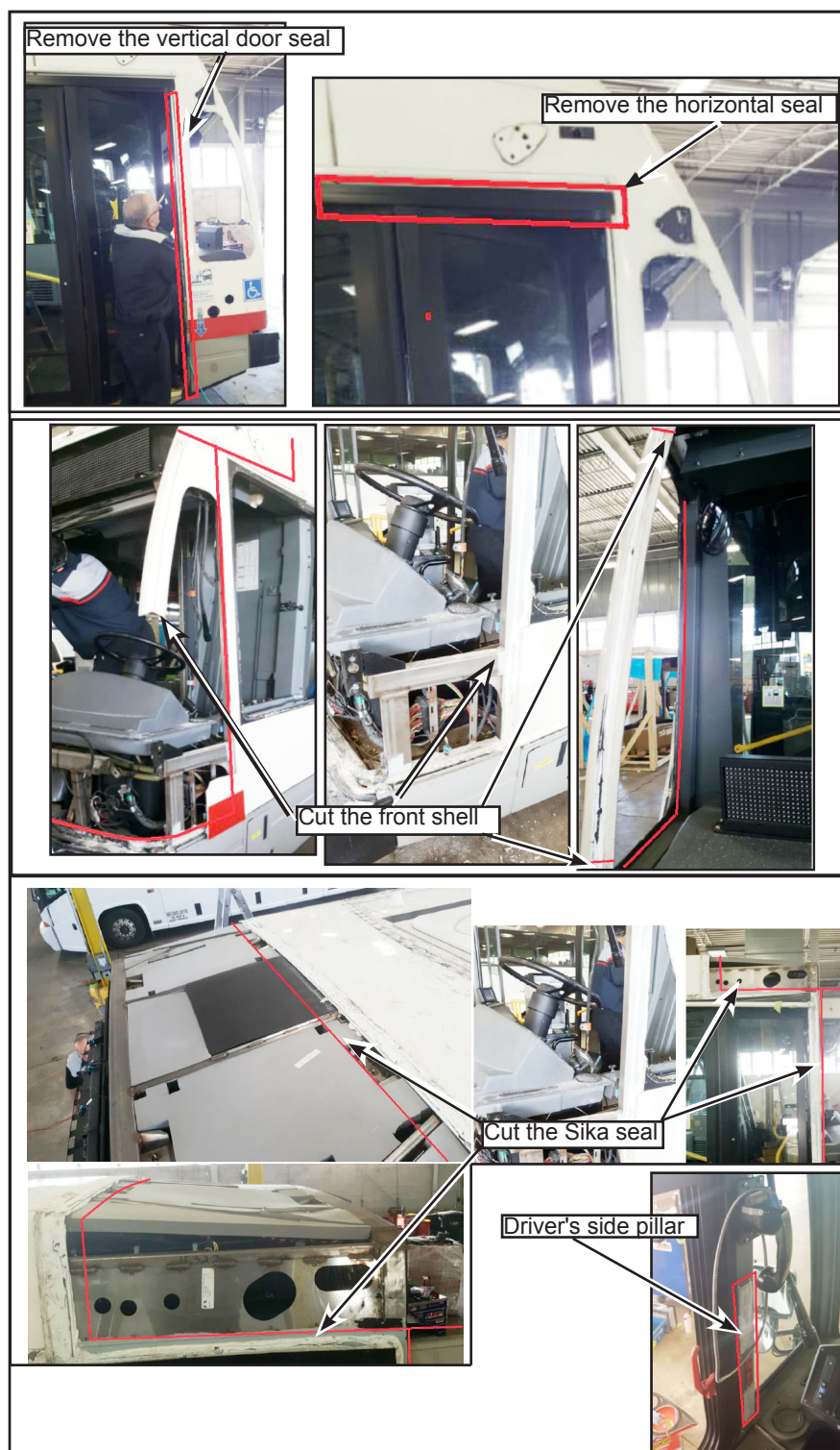
Figure 21 - Remove the Front Shell
