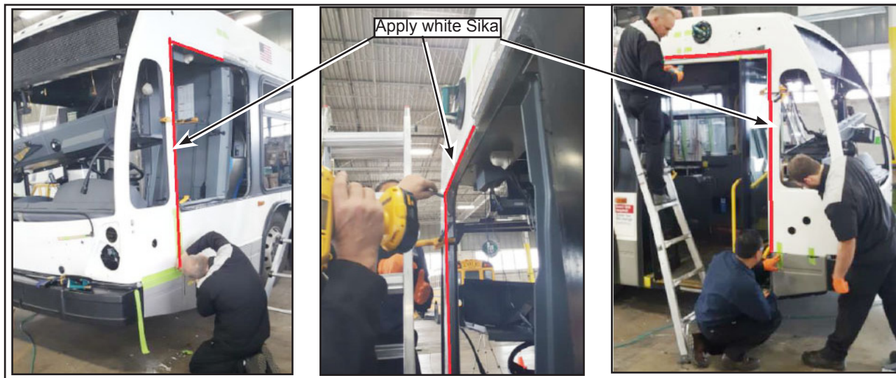
Figure 30 - Apply Sika Between the Front Shell and the Bus Structure
