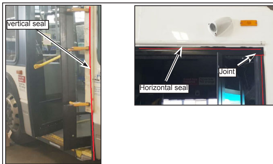
Figure 46 - Install Door Seals
