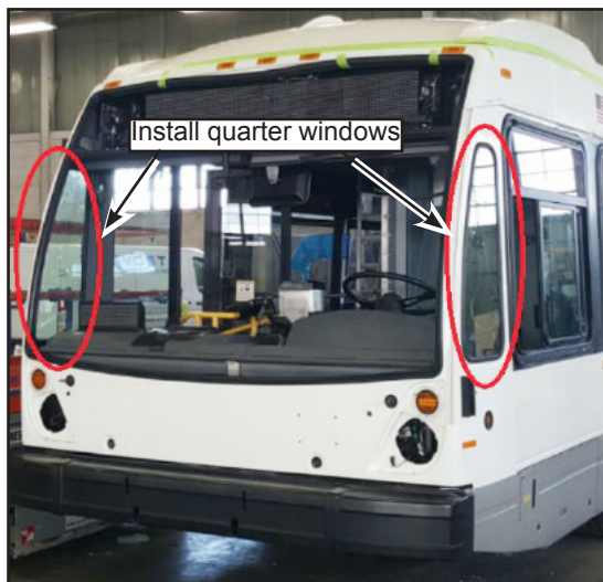
Figure 36 - Install Quarter Windows
