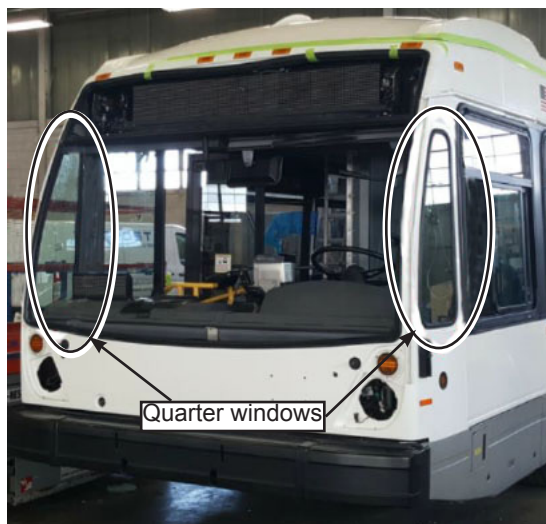
Figure 14 - Remove the Quarter Windows
