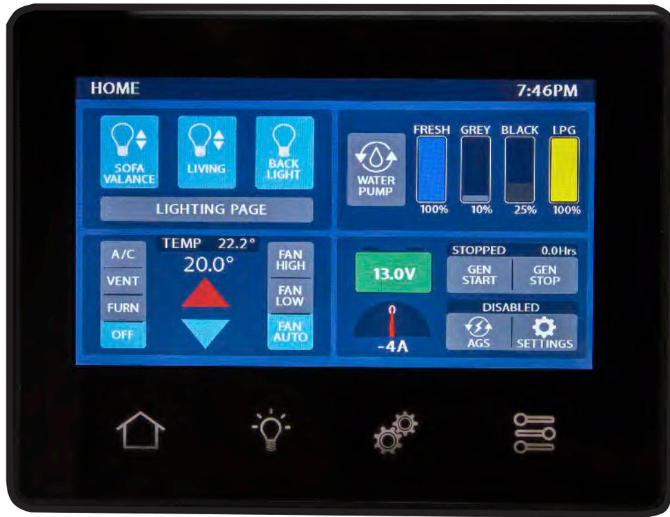
The item on the display is 'on' if the control switch is displayed in light blue.
