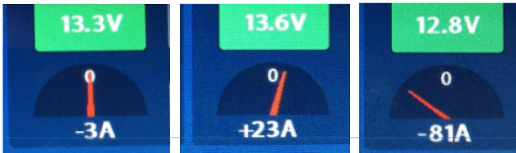
The loss/gain amperage meter will allow you to monitor the amount of draw on the coach batteries. This allows the user to balance out the power use, to enhance the dry camping experience. The three examples above show a dry camping situation with little to no sun, plugged into shore power and dry camping operating the microwave on the inverter. The amperage readings will vary depending on the number of appliances in use, and the amount of charge going into the coach.
