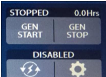
From these switches you are able to start and stop your generator. Touch and hold the button to start the generator. There will be a slight delay before the starter engages.
