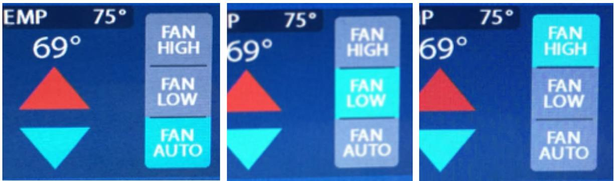
The FAN HIGH, FAN LOW and FAN AUTO are used to control the air conditioner fan speed only. These controls will not affect the roof vent or the furnace fan speeds.
