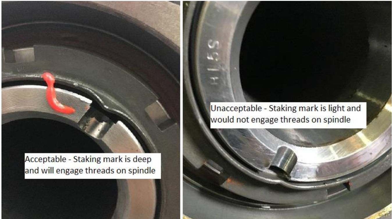
Figure 3: Exemplar staking marks
