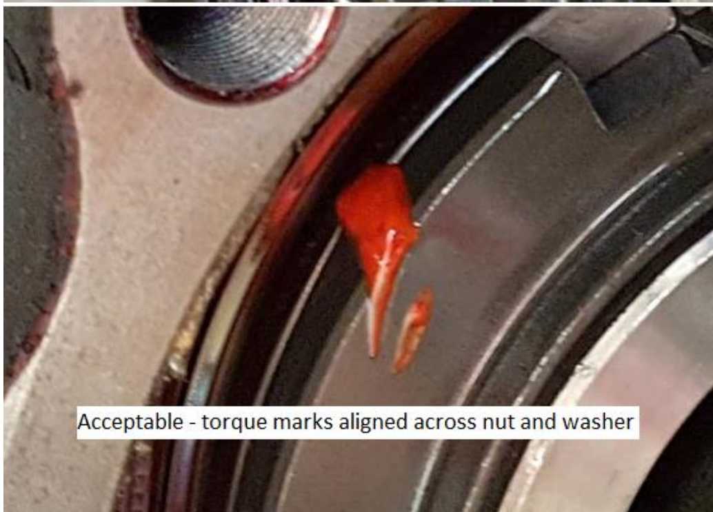
Figure 2: Exemplar spindle nut torque marks
