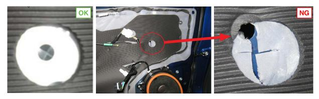
If inspection shows areas where the foam has been crushed by the corresponding retaining clip boss on the inside of the door trim panel, CAREFULLY trim the crushed foam away using a small, sharp scissor, leaving just the thin plastic vapor barrier as shown below. DO NOT try to re-position or separate the foam sealing cover from the vapor barrier as it will get damaged.
