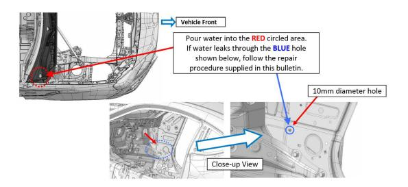
6. After confirming the leak presents as described above, the repair will be to apply additional sealer to the area as described in the illustrations below. Use a large, long, flat-blade screwdriver as the sealer applicator, working through the 27mm cowl area drain "Work Hole".
