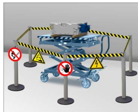
Restricted area for HV battery
