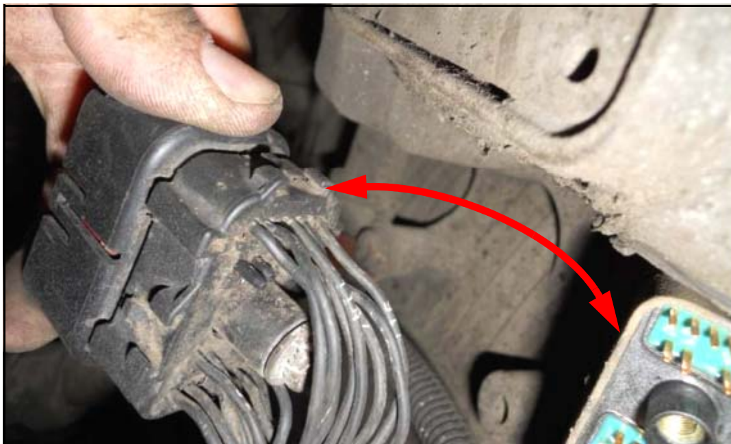
Figure 4. Transmission harness connector removed from the interface port.
