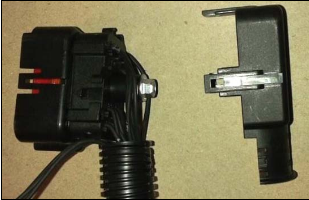
Figure 7. Back cover removed.
