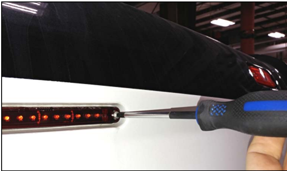
Figure 2. Installation of high mount brake light.
