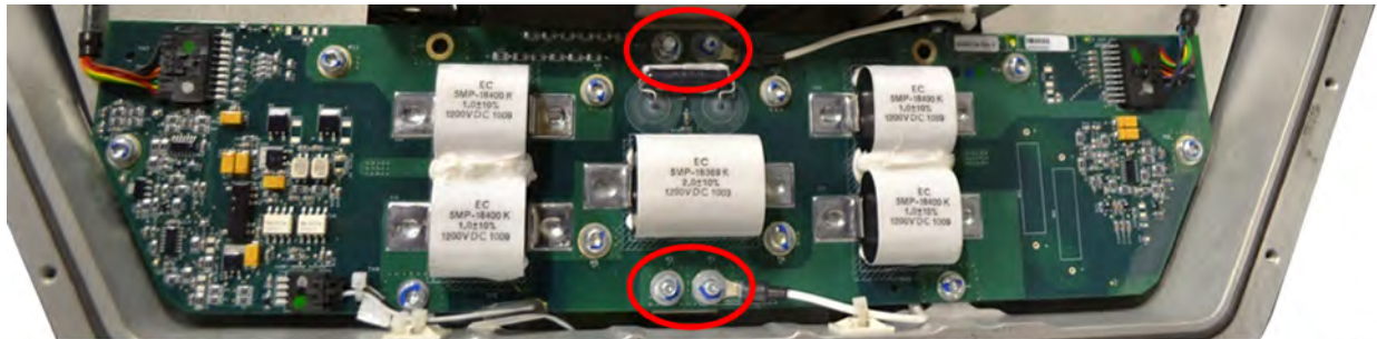
Figure 41. HVIL Circuit Card – Four (4) Mounting Nut/Washer Locations (M5)
