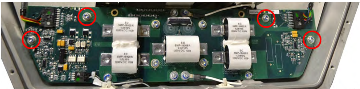
Figure 12. HVIL Circuit Card – Four (4) Mounting Screw Locations (M5 x 22mm)
