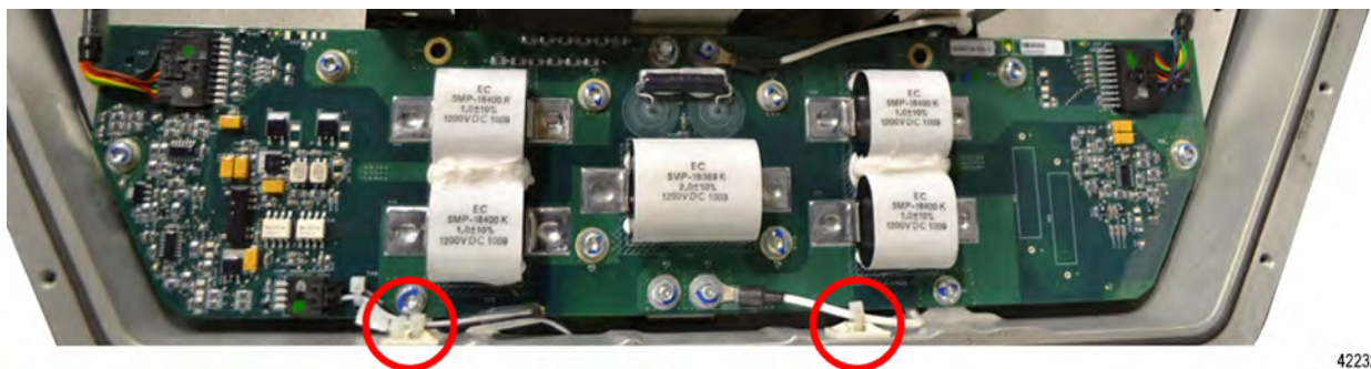
Figure 42. HVIL Circuit Card – Two (2) Wire Tie Locations
