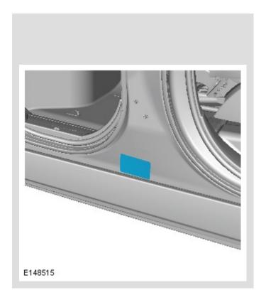
Remove the existing VIN Certification Label attached to the left B-Pillar.
