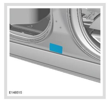
Install the new VIN Certification Label to the left B-Pillar in the identical location of the removed label.
