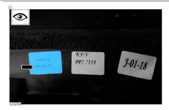
Visually inspect the date printed on the label attached to the new A-Pillar moulding.
