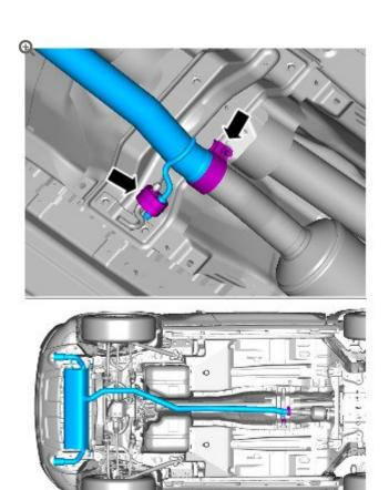
Install the exhaust system rear section.
