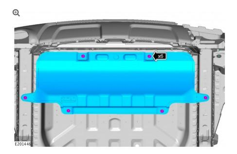
Install the new exhaust system rear heat shield and fasteners.
