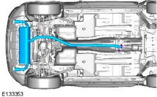
Remove the exhaust system rear section.
