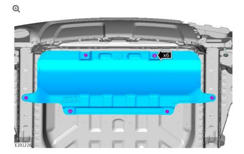
Remove and discard the exhaust system rear heat shield and fasteners.
