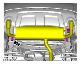
Remove the exhaust system rear mountings.
