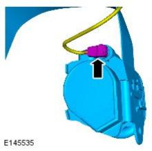
Remove the second row seating outer right seatbelt retractor.
