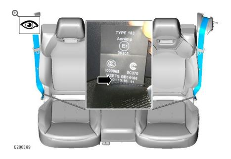
Visually check the date codes of the second row seating outer seatbelt labels.
