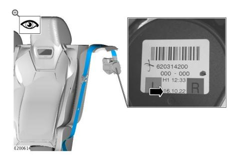
Visually check the second row seating outer left seatbelt retractor label date.
