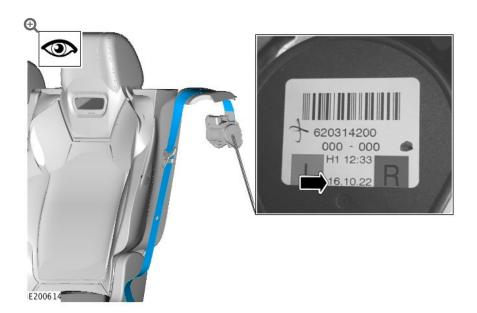
Visually check the second row seating outer right seatbelt retractor label date.
