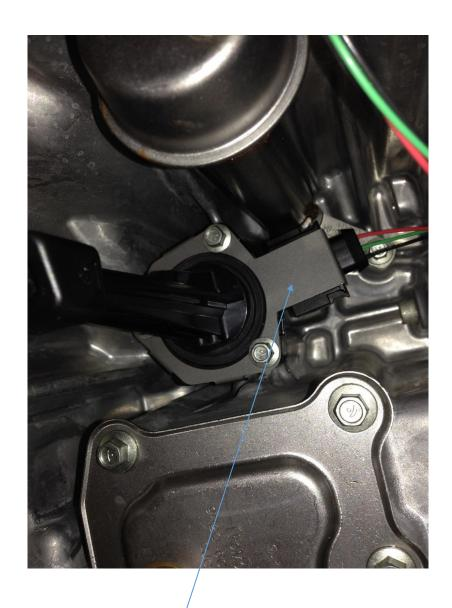
Close up of retainer plate in place over the oil level sensor
