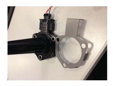
View of retainer plate with the oil level sensor behind it.
