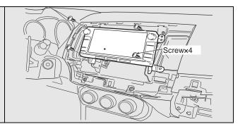
6. Reinstall the vehicle parts in the following order: Center panel, C, B, and A as indicated.
