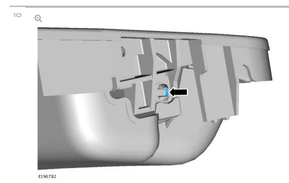
Apply a small amount NyoGel® 774L grease to cam latch hole, rotate the cam latch to distribute the grease, and wipe off any excess.
