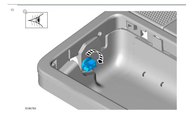
Rotate the cam latch through 360 degrees while visually inspecting it for possible damage.
