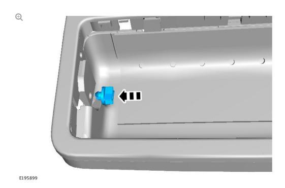
Apply a small amount NyoGel® 774L grease to the cam latch hole in the front overhead console frame and install a new cam latch.
