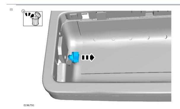
Remove and discard the damaged cam latch from the front overhead console.
