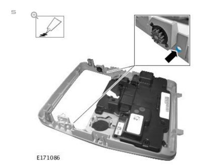
Apply NyoGel® 774L (or equivalent) into the hinge pin holes.
