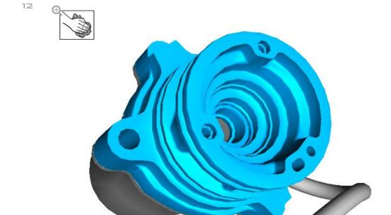
Using an air blow gun, make sure that the breather is clean and free from foreign material.
