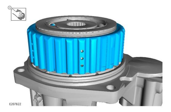
Clean the Active On-Demand Coupling using lint-free cloths and an air blow gun.
