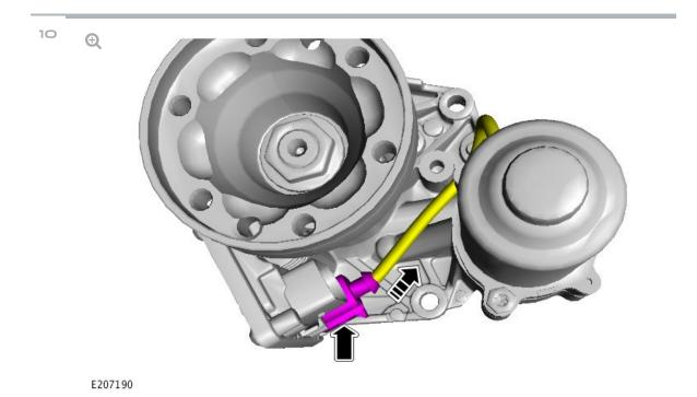
Disconnect the electrical connector from the Active On-Demand Coupling.
