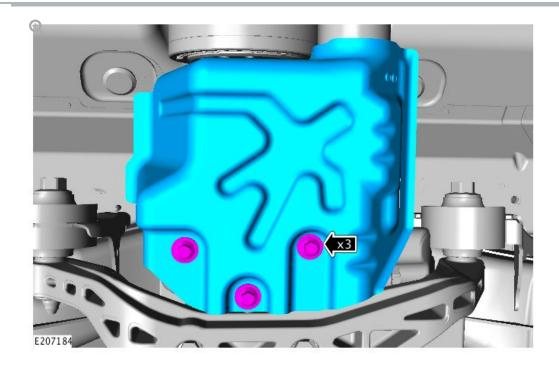
Remove the Rear Drive Unit (RDU) heat shield.
