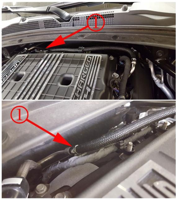
These pictures above shows the chassis fuel feed pipe for the LT4 supercharged ZL1 Camaro. On LT1 Camaro and LT4 CTS-V this line would have a jumper line with quick disconnects at both ends. One end will connect to the chassis line and the other to the high pressure pump feed line.
