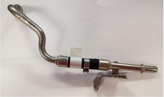
The line above is the fuel feed pipe for Corvette, truck and SUV. This line connects the chassis fuel line to the high pressure fuel pump.
