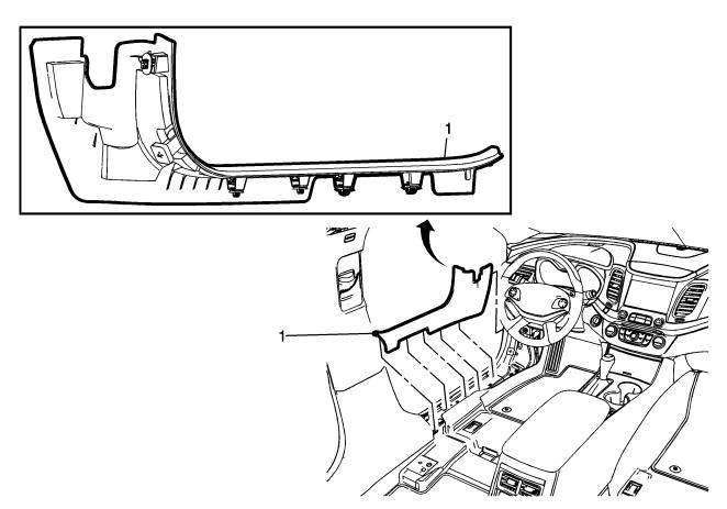
1. Remove the drivers front side door sill garnish molding (kick panel) (1). Refer to Front Side Door Sill Garnish Molding in SI.
