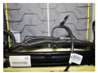
6. Separate the wiring harness from the forward seat frame.
