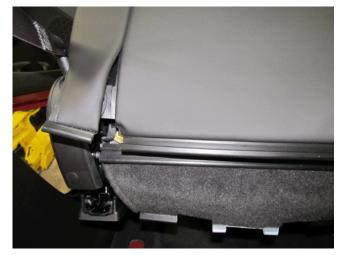
3. Disengage the drivers side seat back cover lower center and inboard J channel from the seat back frame.
