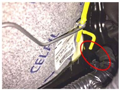
Note: When installing the tie straps, ensure they are installed in a position where they will not damage the seat cover.
