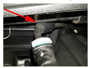
3. Re-install the foam sleeve to a location that will keep the pipe from contacting the cowl panel as illustrated above.
