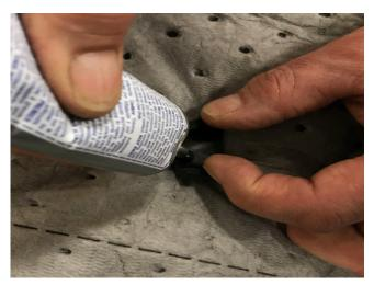
2. Apply weatherstrip adhesive or equivalent to the foam sleeve to prevent the sleeve from moving again.
