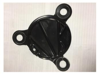
GM engineering is requesting that every time a wheel bearing is replaced that a dust shield is ordered for that side and the opposite side as well.
