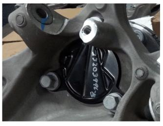
The newly installed dust shield will protect the new bearing and prolong its life-span and the dust shield on the opposite side will prolong the old wheel bearing.
