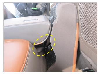
Release the 60% seatback by carefully cutting the rear center seat belt, then replace the rear seat center shoulder belt assembly. Easier access to the seat belt can be attained from the passenger side of the vehicle.
