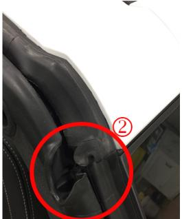
**Note:** Shown in the illustrations above are examples of the old design (1) and the latest design (2) removable roof weatherstrip.
