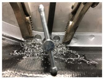
8. Using a 5/16th (8 mm) drill bit, drill two holes in the areas with the most overlap.
