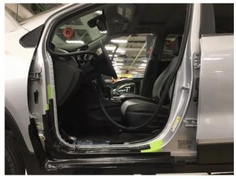
6. Mask off the areas illustrated above to ensure that none of the painted surfaces are damaged.
