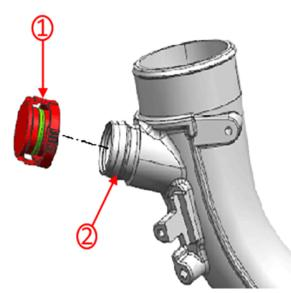
5. Install the block off plug (1) onto the turbocharger bypass port (2).
