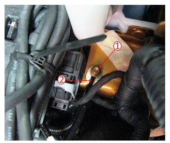
21. Install the PCV heater wiring harness ground (2) to an existing ground located at the frame stud (1).
