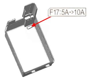
22. Install the UEC sticker onto the backside of the fuse block cover and in the owners manual under Engine Compartment Fuse Block.
