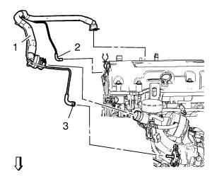
4. Remove and discard the Positive Crankcase Ventilation Hose/Pipe/Tube (1) and vacuum line. Refer to Positive Crankcase Ventilation Hose/Pipe/Tube Replacement in SI.
