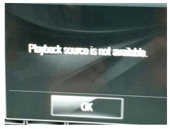
If you can't perform USB programming first because of the "playback source is not available" message above remaining on the screen and preventing you from continuing, skip to SPS programming and complete it first instead. Once the SPS programming is complete, it should repair the pop up message so you can then complete USB programming but this should only be performed in this order if the "playback source is not available" message remains displayed.
