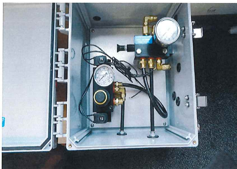
Part #024-59003 Alkon Rear Lift Axle Control, Dual Solenoid, Regulated Lift
