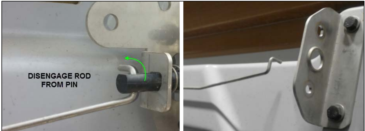
FIG.13 DISENGAGING ACTUATING ROD FROM LATCH PIN
