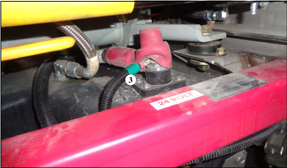
Figure 2. Lower cable from circuit breaker routed to 24V power stud.
