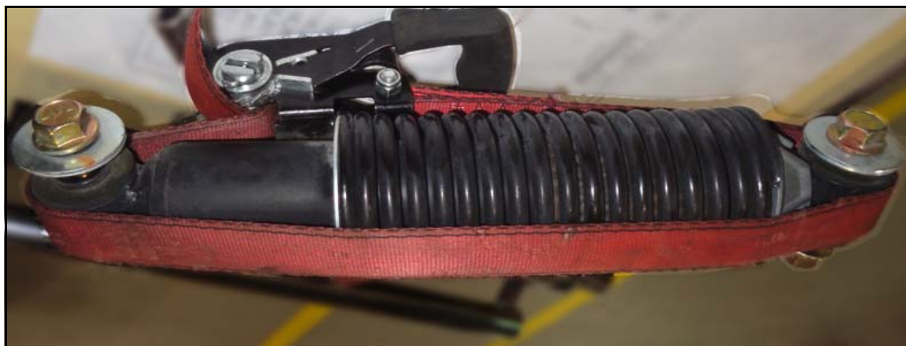
Figure 28. Reference photo of ratchet strap compressing tensioner.
