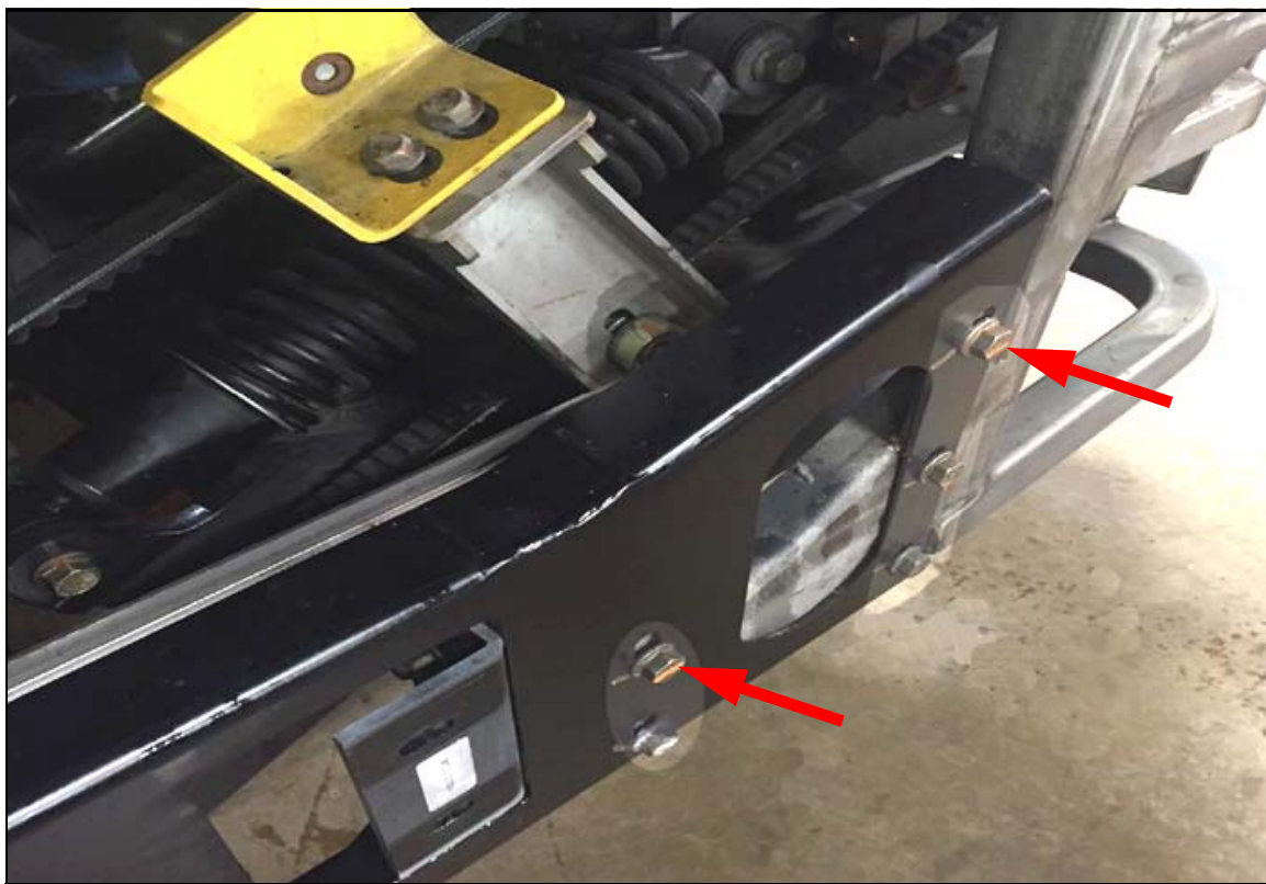
Figure 9. Tie bar plate installation.
