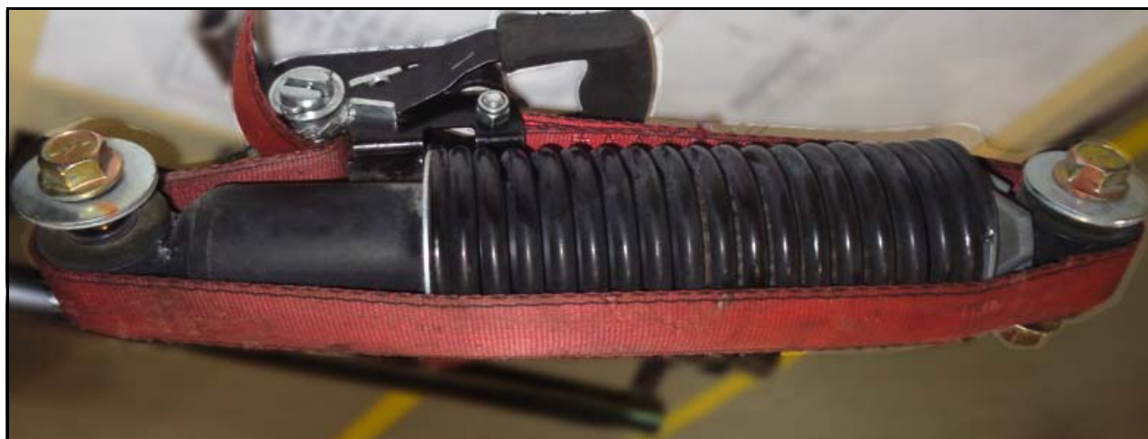
Figure 13. Reference photo of ratchet strap compressing tensioner.
