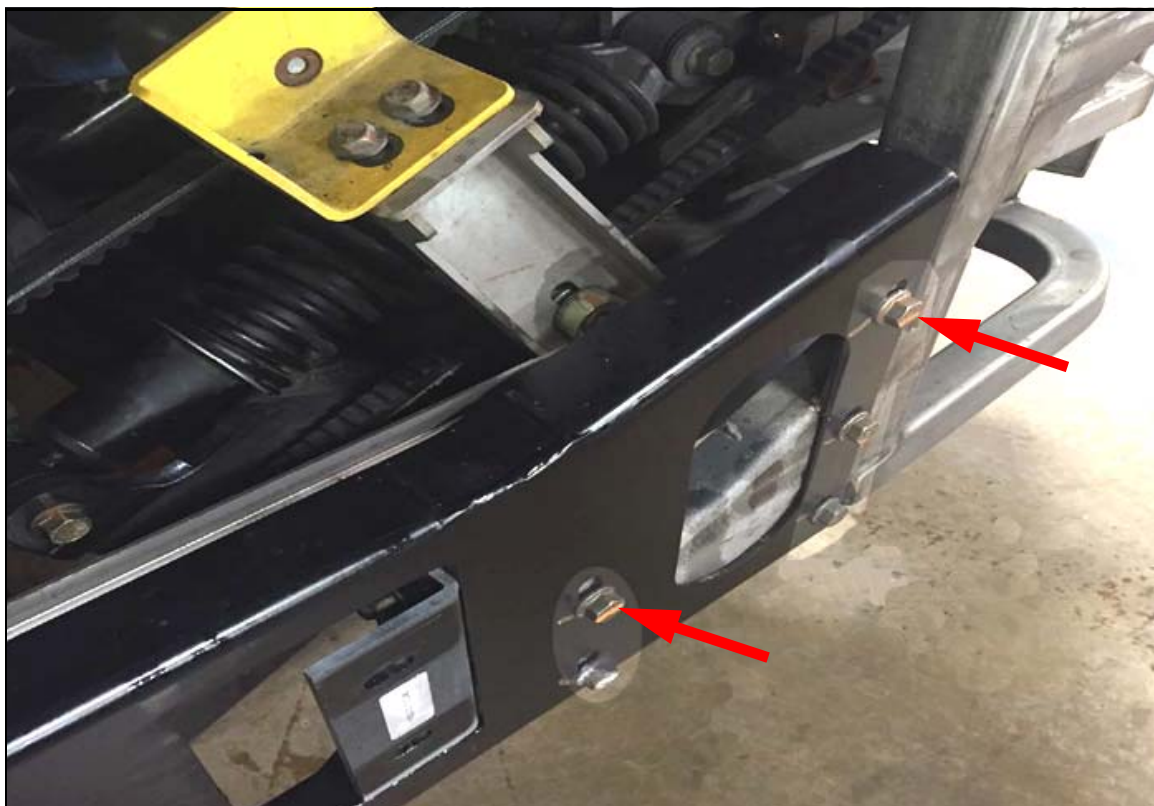
Figure 24. Tie bar plate installation.
